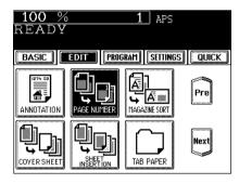
Select the orientation (Short edge or Long edge) and position of the page number to be printed.
